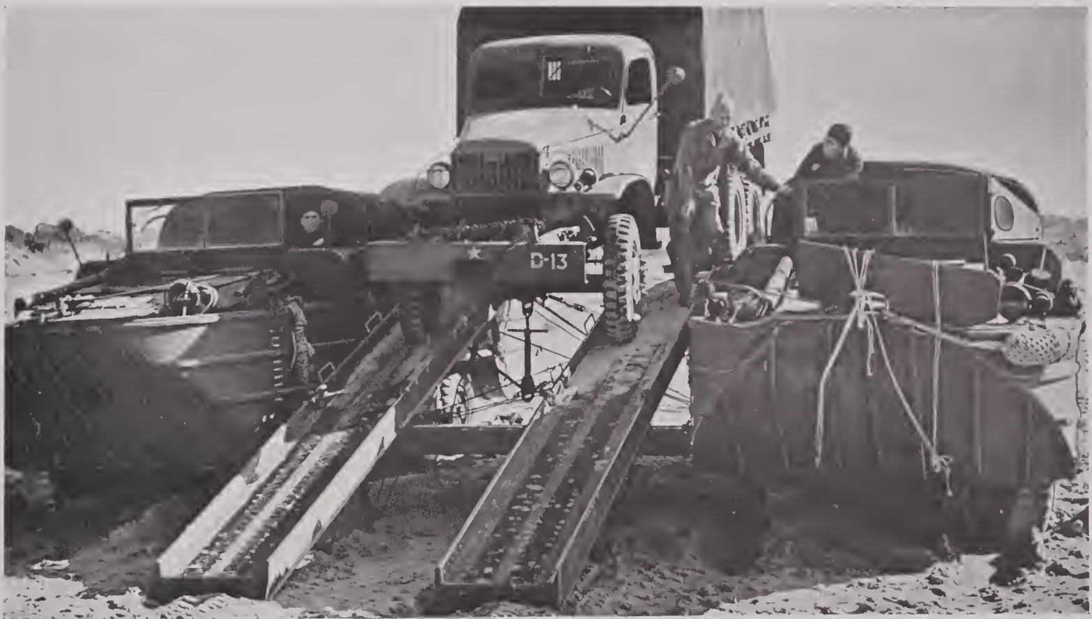
FIGURE 69. Army 6x6 truck backing up treadway for dry ferry test off Fort Story, Virginia.
